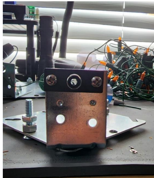
Completed Radial/Connection Plate
