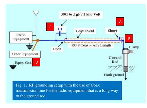
Installation of the RF suppressor -
