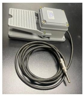
Within a few minutes, I discovered a reasonable foot switch available from Amazon for around \$20. I ordered it and as soon as it arrived, disassembled it and checked out the internals. The pedal is hearty and cast aluminum construction and internally has a sturdy switch that is operated by the pedal operation. Some cheaper switches simply have two metal plates that make contact, but this is not that type, and you should avoid this type of noisy switch as well.
