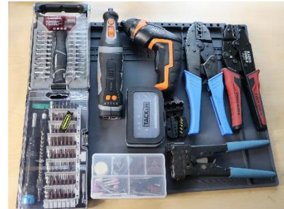
Precision Screwdriver sets, Rotary Tool, Battery Screwdriver, Ratcheting Crimp Tools and Dies
