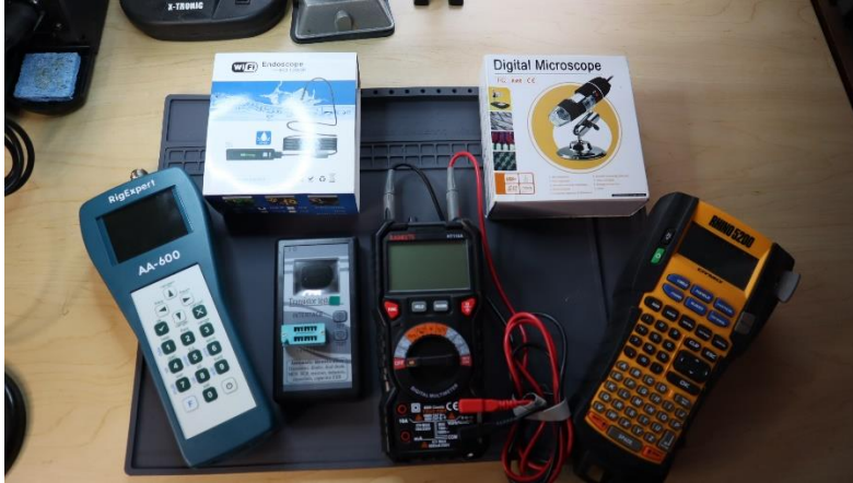
Rig Expert AA600, DROK Component Tester, Kaiweerts Multimeter, Dymo Labeler, Mini-borescope and Microscope
